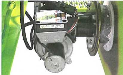
340,000 BTU Diesel Material Tank Burner
